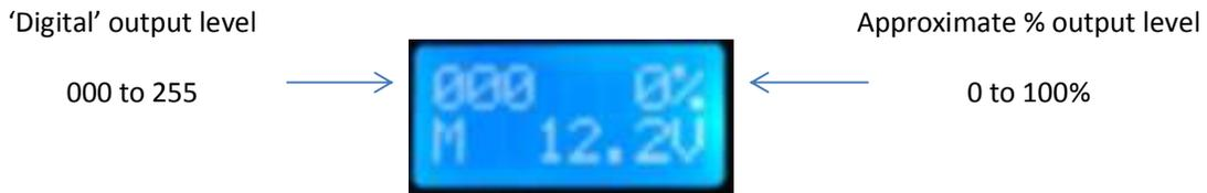
The LCD display will also indicate the actual supply voltage present, bottom right, and the source of the supply, bottom left. The display will indicate BX to warn the user that the battery voltage has dropped below 7V and will require charging soon.
