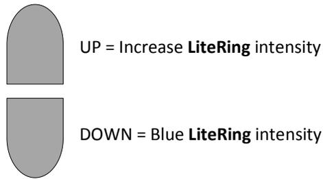
The light output can be very finely controlled in 256 discreet steps (i.e. values of 0 to 255).
